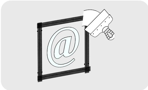
10 - Remove the protective film when the paint is still wet.
