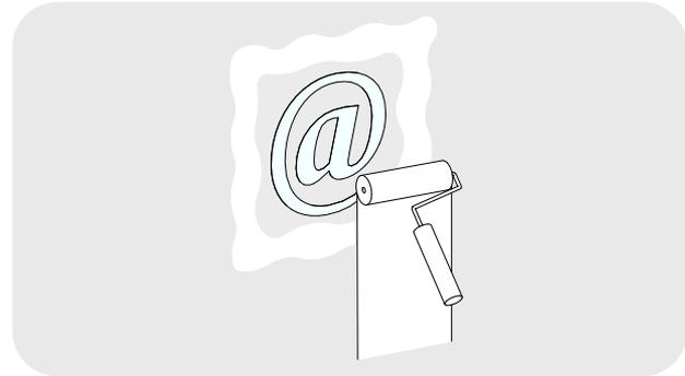
8 - Apply the adhesive mesh (not supplied) along the joints and plaster to get an uniform and leveled surface.
