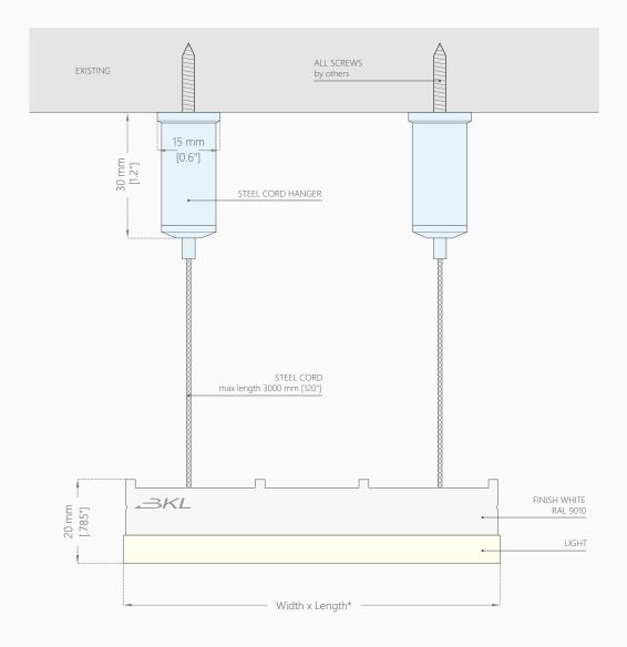
\* Width from 15 mm to 203.2 mm (from 0.6" to 8"). For different widths see Magic Cloud.
