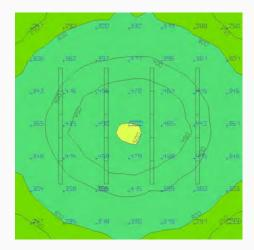
\* EXAMPLE of a room 3x3 x h. 2.70 meters (118"x118" x h. 106") with 4 lamps 50.8 x 1524 (2"x60")
