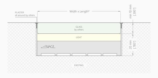
\* Width from 15 mm to 203.2 mm (from 0.6" to 8"). For different widths see Magic Cloud.
